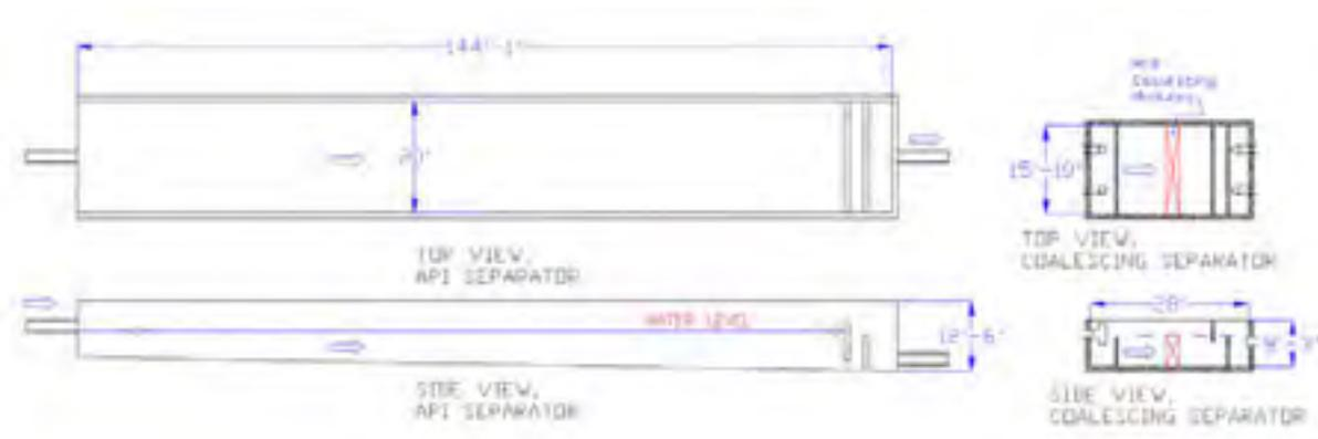
Figure 9: Comparison of API and Coalescing Separators
