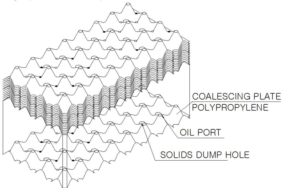
Figure 6: Typical Coalescing Module
