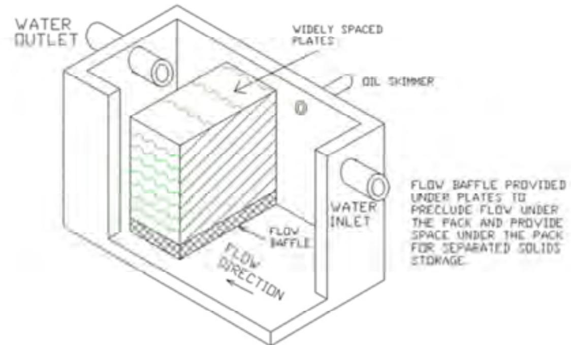
Figure 4: Inclined plate separator
