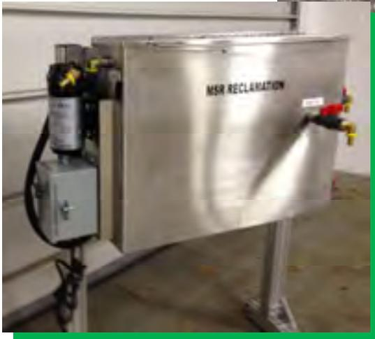
Machine tool coolant Separator: capacity 0.5 US gpm (0.3 lps)
