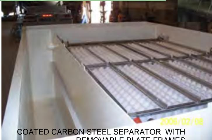
COATED CARBON STEEL SEPARATOR WITH
