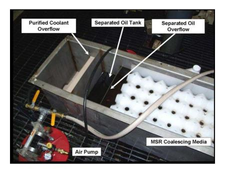
Eventually enough oil built up in the front of the system to begin flowing under the oil tank and appeared in the outlet end overflow. It was suspected that the captured oil was of much higher density than is encountered in most facilities. Subsequent testing indicated that the specific gravity of the captured oil is 0.93, consistent with a very heavy lubricating oil. The coolant specific gravity was found to be approximately 0.99.
